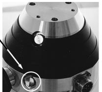
Remove the syringe and reassemble the lubricating plug equipped with its new o-ring.
